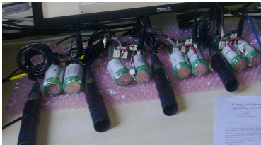
(a) Four sensor nodes with an unidirectional infrared barrier attached
