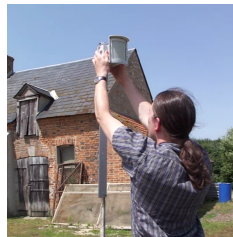
(c) Deploying a 16-beam infrared sensor
