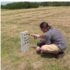
(a) Deploying a Thales infrared barrier
