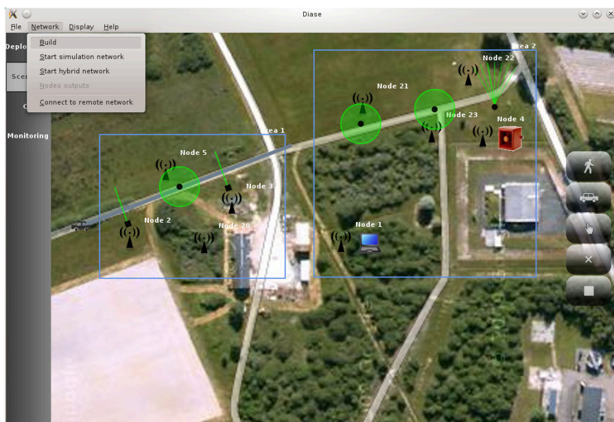
Figure D.2: Running options for the network (building, running the gateway, running a simulation)
