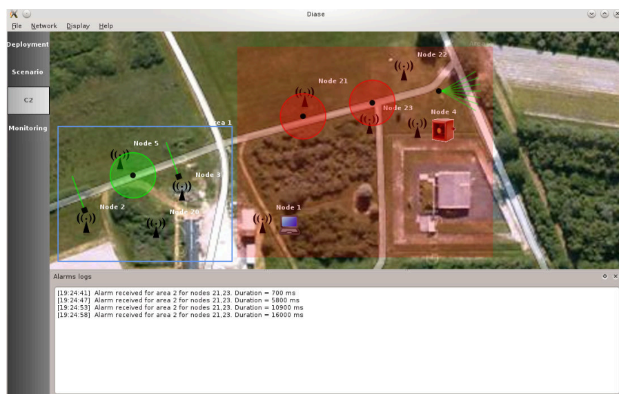
Figure D.8: Command & Control mode : Visualisation of an alarm in an area along with which sensors participated in it
