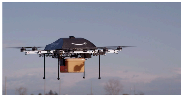
Figure 7.3: Amazon Prime Air: A commercial drone delivery proposed by Amazon [15]
