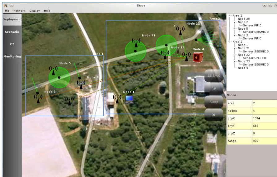
Figure D.1: Deploying a network using Diase
