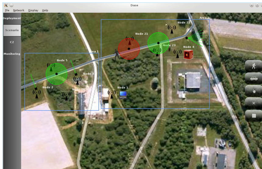
Figure 3.9: Screenshot of Diase running an intrusion scenario in real time and injecting simulated events to the emulated wireless nodes.
